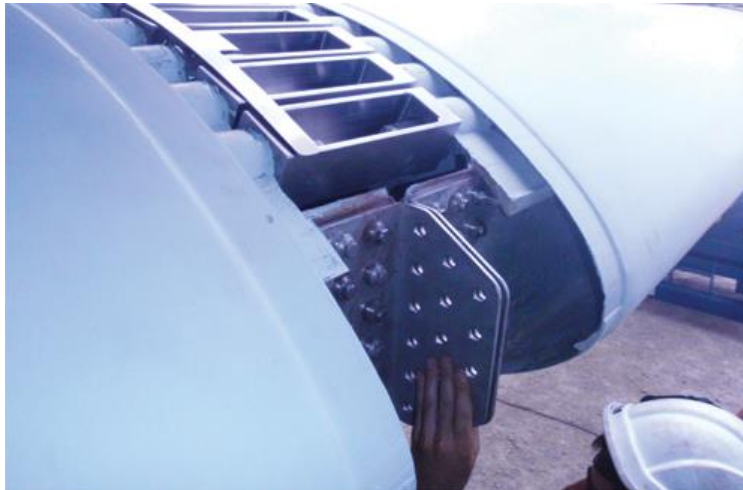
Figure 5-9. Jointed wind turbine rotor blade
